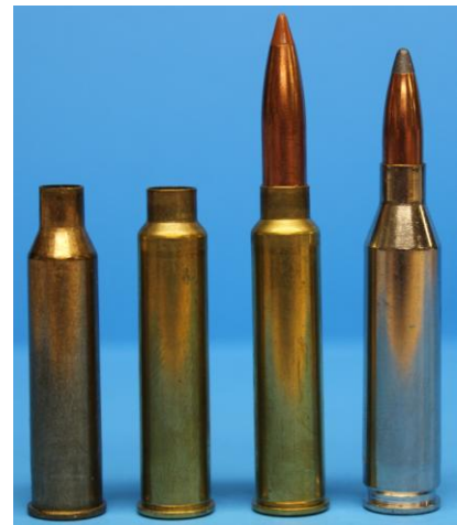
From left to right, the .225 Winchester case serves as the parent for the 6.5 JDJ shown to its right. A 6.5 JDJ loaded to an OAL of 2.900" with a 120 Gr. Nosler Ballistic Tip. A .243 Winchester round is included for comparison.
