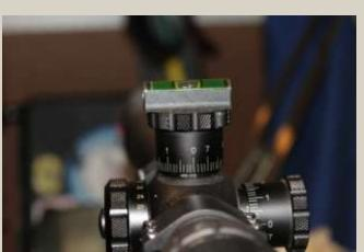
the flat surface of the scope base, which is attached to the rifle, to level the rifle. The smaller level is then applied to the elevation
