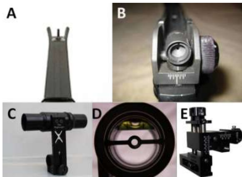
The sights found on the service and match rifles are shown. In panel A, the standard service rifle front sight is shown with a narrow post. In panel B, the modified rear sight is shown with a corrective lens in the hood. Panel C and D show the Stallings Machine "Rightsight." The iris is adjustable. In panel E, the Phoenix side-mount rear sight is shown.
