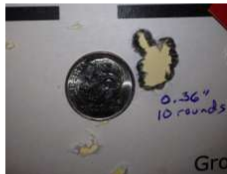
This 10-shot group was fired at 100 yards using the Berger 105 Gr. BTHP bullet with 29.1 Gr. Hodgdon Varget and a GM205M primer in Hornady cases. Note that the single high left shot in the group was called "out" by the author as soon as it was fired.
