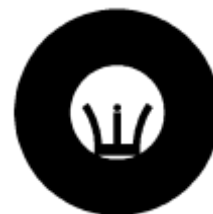
The sight picture through the rear peep sight of the AR15 with the post front sight centered underneath the target is called a "6 O'clock Hold."
