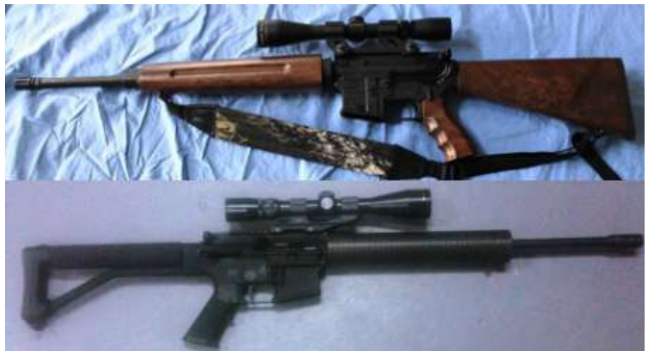
My rifle (top) and Dan's rifle (bottom) demonstrate the versatility of the AR-15 component system. Dan's rifle was built on a carbine-length barrel that is free floated under the tube style hand guard. The skeletonized buttstock also significantly reduces the weight of the rifle.
