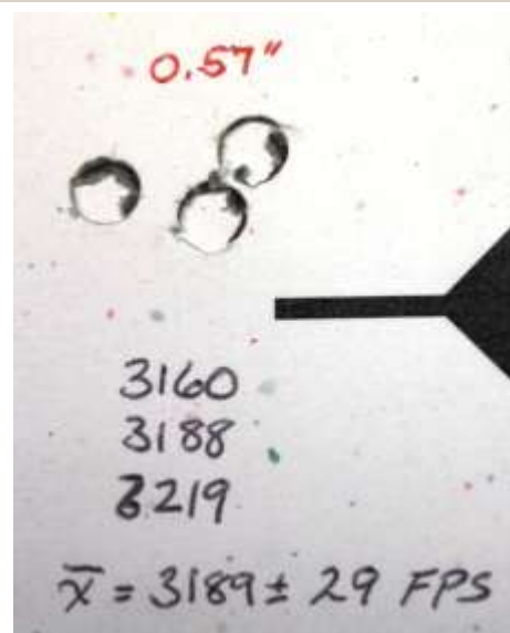
A nice 0.57" 3-shot group was fired using a 140 Gr. AccuBond over 68.5 Gr. IMR7828SSC, CCI-250 primers in WW brass for a COAL of 3.316". Muzzle velocity is 3189 \pm 29 \text{ FPS} .
