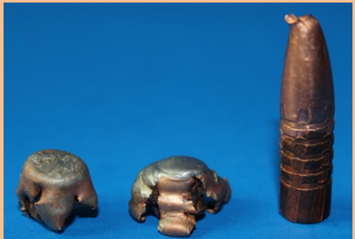
The Tale of Three Bullets: (from left to right) the 160 Gr. Nosler Partition fired from the XP-100 and recovered from the off-side of the Kalahari Gemsbok and the 175 Gr. Nosler Partition fired from the M77 and recovered from the off-shoulder of the Blue Wildebeest both performed exactly as advertised. However, the 300 Gr. Barnes TSX fired from the PH's .375 H&H Magnum has barely been deformed and did not expand, essentially acting as a solid bullet.
